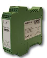
The PSESB Series is a range of inrush current limiters designed to protect against unintended fuse or circuit breaker activation caused by peak currents. The benefits can result in reduced cable cross section and the use of smaller and faster circuit breakers. These are not simple NTC devices and feature current control circuits with integrated bypass relays.
